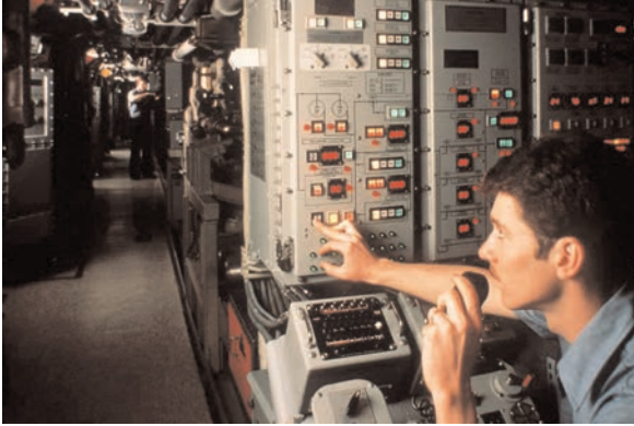
Missile Control and Monitoring Panel (CAMP) Watch on a US Trident submarine 6
